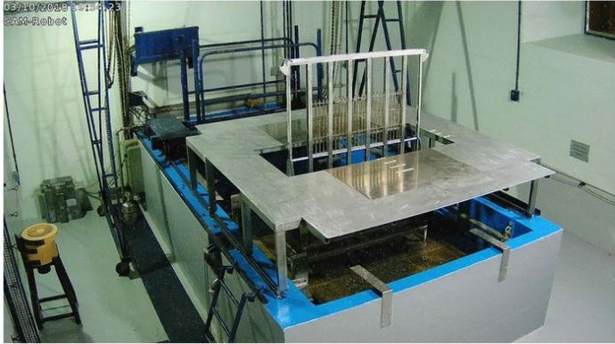
*Calliope source rack within the irradiation cell (picture acquired by a remote camera).*
